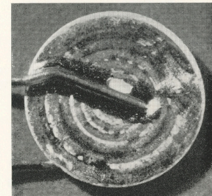
Figure 4. Defective ceramic capacitor detected by a very unstable 3rd harmonic voltage reading. The tinned surface has annular irregularities and a big hole at the terminal.
